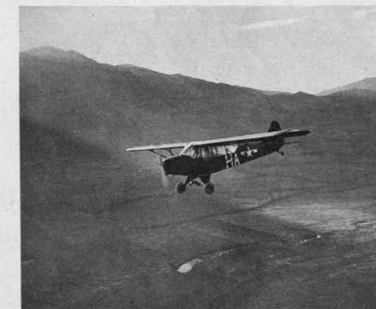
Turned-up nose with uncowed engine is typical of the L-4. Slow speed permits the use of tall radio wand. Pilot and observer usually sit tandem in large cockpit enclosure which fairs into the fuselage.
